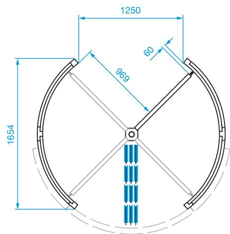
Concrete Base to specification at least (cube) 30N/mm<sup>2</sup> of resistance. Base to be flat and level to +/-5mm over footprint area. Dimensions to be > 2250 x 2250 x 150 deep min. (units in mm).
