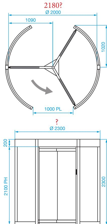
Concrete Base to specification at least (cube) 30N/mm<sup>2</sup> of resistance. Base to be flat and level to +/-5mm over footprint area. Dimensions to be > 2250 x 2250 x 150 deep min. (units in mm).
