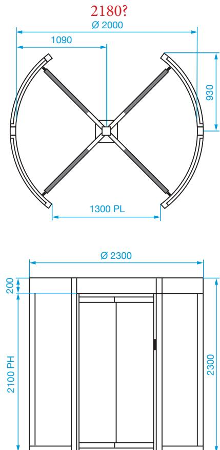
Concrete Base to specification at least (cube) 30N/mm<sup>2</sup> of resistance. Base to be flat and level to +/-5mm over footprint area. Dimensions to be > 2250 x 2250 x 150 deep min. (units in mm).
